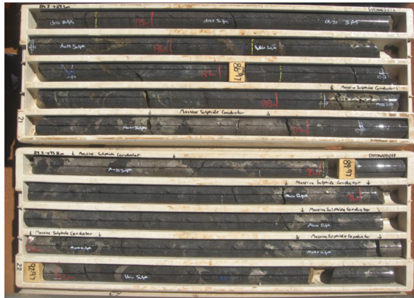
Figure 4 – DD13WOD017 from depth 84 to 93 metres: image showing massive to semi-massive pyrrhotite hosted within a sulphidic pyroxenite and gabbronorite.
