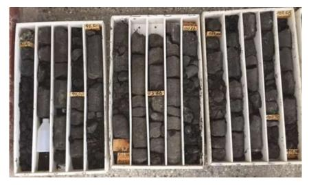
Photo 2 - Black Sand in Borehole PNN-VI-DW-02 from 92-107metres depth.
