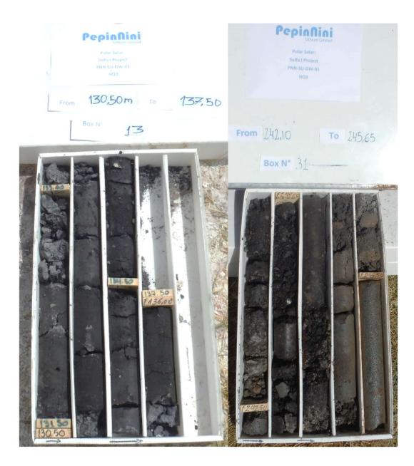
Photo 4 Black Sand in PNN-SU-DW-01 from 130.5-137.5 metres and Breccia unit 241.65-245.65metres
