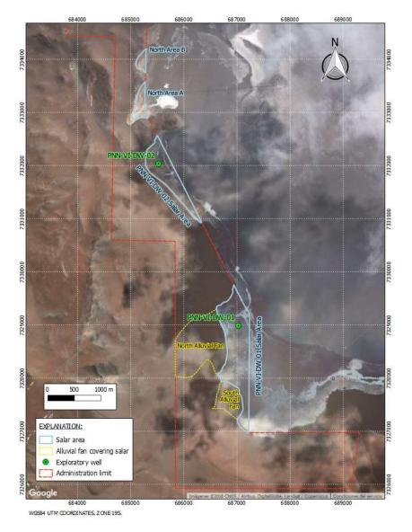
Figure 3 - Borehole Locations and Polygons used for Resource Calculations - Salar del Rincon
