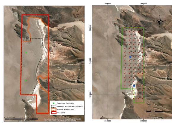
**Figure 3a:** Incahuasi salar showing location of two planned drillholes (green dots) and potential Resource area **Figure 3b:** Revised drill hole locations (blue dots) and previous TEM geophysical survey points (red dots)
