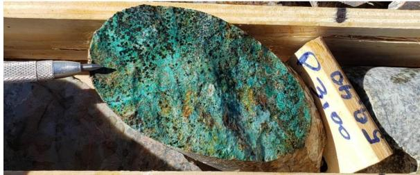
Drill core from hole PNSI22-002 at 59.4m showing quartz-biotite-magnetite veins with Cu-Fe oxides
