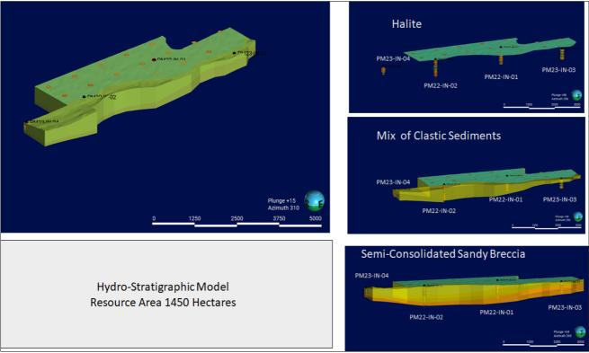
Figure 2: Hydro-Stratigraphic units and model used in Resource Estimate, Sisifo licence, Incahuasi salar
