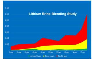
**Figure 1** - Lithium ion concentrations against time for mix and individual brines through the evaporation process.
