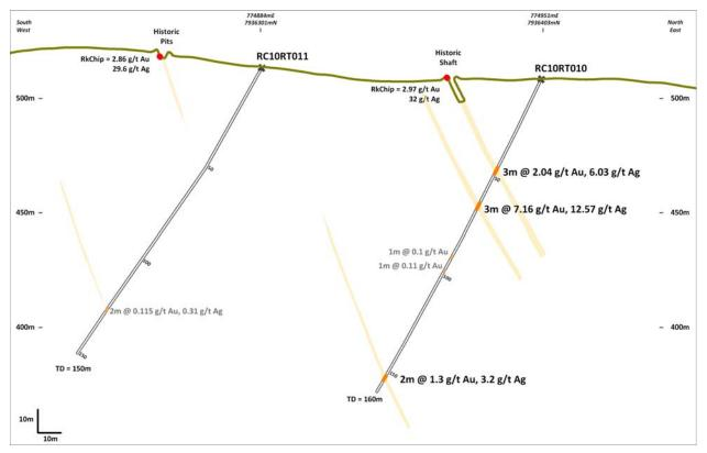
Figure 3. Diagrammatic Cross Section Boreholes RC10RT010 and RC10RT011
