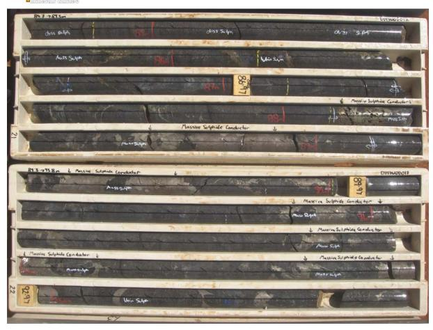
**Figure 3:** DD13WOD017 from depth 84 to 93 metres: image showing strongly disseminated and massive pyrrhotite hosted within a sulphidic pyroxenite and gabbronorite.
