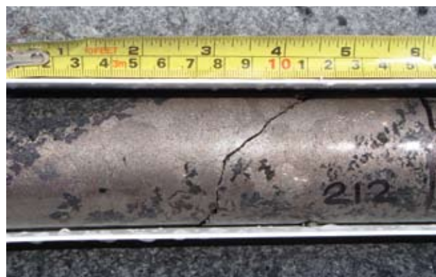
Borehole DD07HAR008: 211.9 – 212.0m. Massive sulphide mineralisation consisting primarily of pyrrhotite with accessory chalcopyrite and pentlandite. Assays: 0.29% Cu and 0.31% Ni
