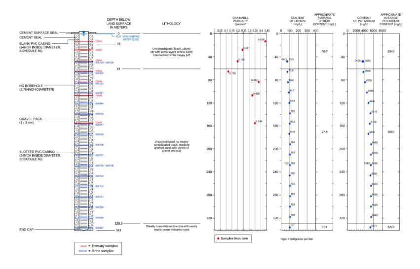
FIGURE 3. SCHEMATIC DIAGRAM OF CONSTRUCTION OF EXPLORATION WELL PNN-SU-DW-02
