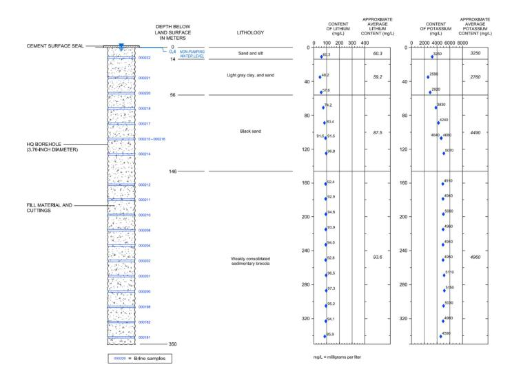
FIGURE 5. SCHEMATIC DIAGRAM OF CONSTRUCTION OF EXPLORATION BOREHOLE PNN-PA-DW-04
