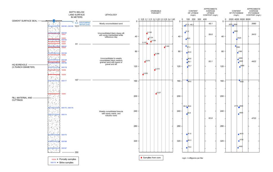
FIGURE 4. SCHEMATIC DIAGRAM OF CONSTRUCTION OF EXPLORATION BOREHOLE PNN-PA-DW-03
