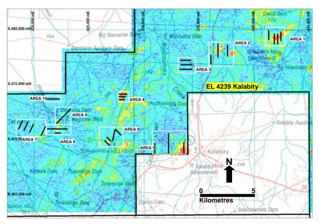
Figure 2: Proposed Aircore Traverses and Target Areas on Uranium Channel Radiometric Image
