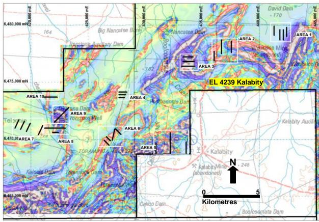
Figure 3: Proposed Aircore Traverses and Target Areas on Aeromagnetic Image
