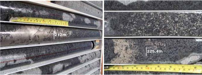
Massive and disseminated sulphides Borehole DD07HAR008
