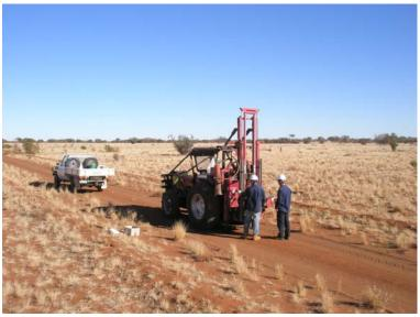
Company vacuum rig collecting bedrock geochemical samples within EL 4048 Mt Caroline
