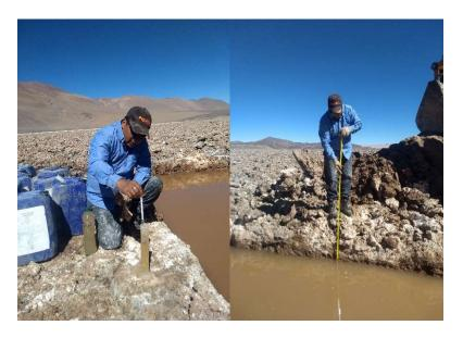
Photo 2 – Brine Sampling Incahuasi Salar conventional evaporation:concentration methodology(Figure 6). The next step will be wind tunnel evaporation testing using the brine samples taken from Rincon and Incahuasi projects.
