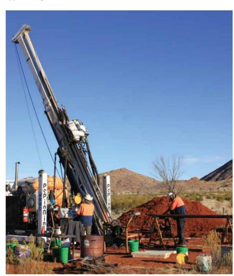
Photo 5 - PepinNini Diamond Core Drilling Rig
