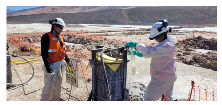
**Figure 4:** Brine sampling from drillhole PM23-IN-03 at the Incahuasi salar, Salta Lithium Project.
