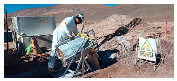
Figure 5: Brines packer testing at drillhole PM23-IN-04 at Incahuasi salar, Salta Lithium Project.
