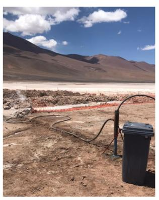
Figure 3: Airlift test of lithium brine flow rate, drillhole PM22-IN-002, Incahuasi salar
