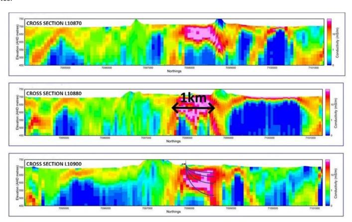
**Figure 7:** Airborne conductivity sections at 300 metre spacing across the Pink Slipper target (red-pink shading) (ASX announcement 31 July 2019) showing the scale of the target (middle cross section) and a schematic design example of the proposed drilling (lower cross section).
