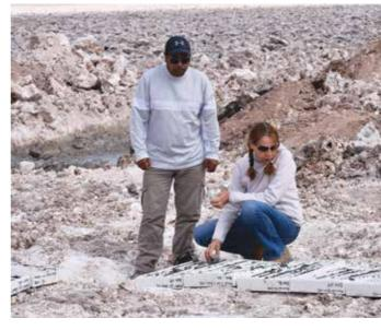
Photo 3a: PepinNini Salta Based Exploration team logging drill core Rincon
