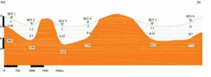
Figure 7: VES Survey Cross Section Rincon Salar - August 2017
