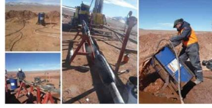
Photo 4: Packer Sampling of Brine from boreholes
