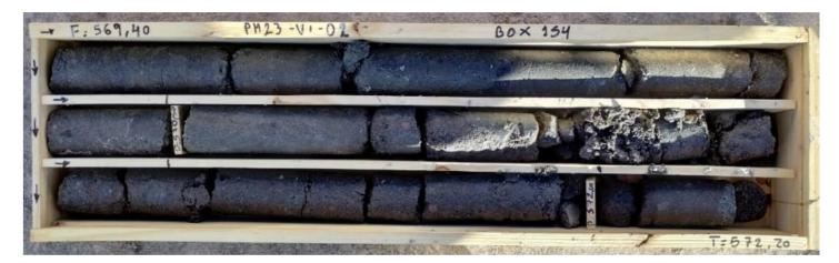
**Figure 3:** Drill core from 569.4 to 572.2m depth in drillhole PM23-VI-02 at Rincon salar (Note: high core recovery and sandy matrix)
