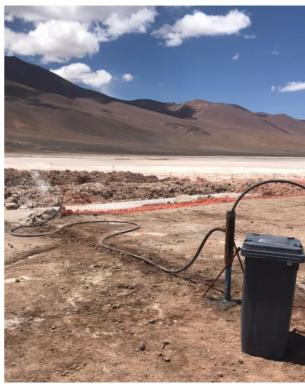
Figure 1: Airlift test of lithium brine flow rate, drill hole PM22-IN-002, Incahuasi salar
