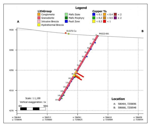
Figure 2: Cross section of drill holes PNSI22-001 showing high-grade Cu surface samples
