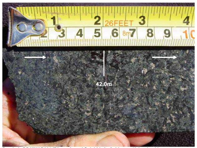
Borehole DD07HAR001 (Disseminated Sulphide in Gabbro at 42.0m depth)
