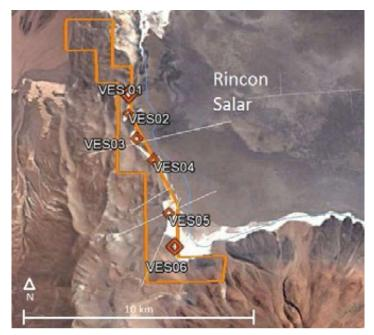
Figure 1 - Geophysical Survey Traverse Location – Rincon Salar
