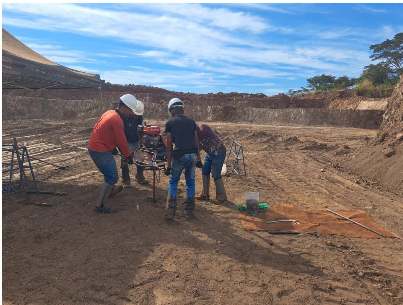
Figure 1: 2 nd phase, shallow auger, drilling program underway at Santa Anna Project. Site is located within test pit for phosphate by EDEM.
