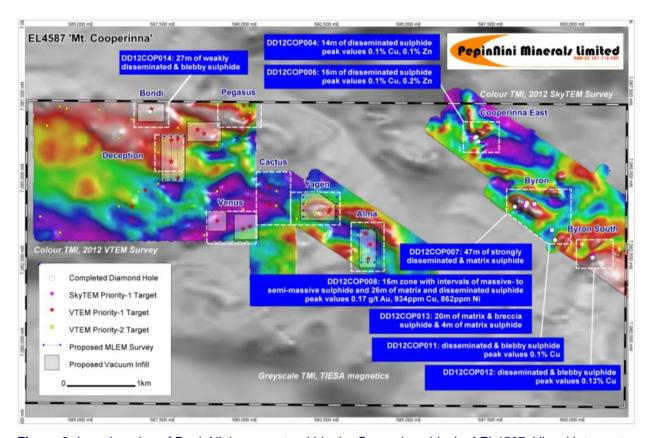
**Figure 2:** Location plan of PepinNini prospects within the Cooperinna block of EL4587. Visual intercepts and peak assay values are provided for selected diamond boreholes
