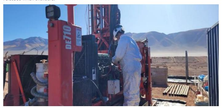
Figure 1: Rig preparation for Mineral Resource drilling at the Incahuasi salar at the Salta Lithium Project
