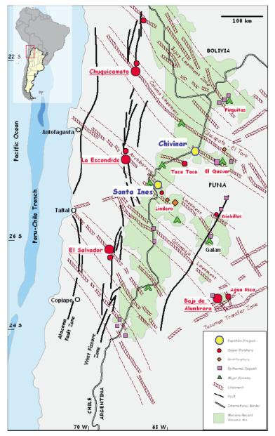
**Figure 2:** Crustal scale NW Lineament control on porphyry-epithermal mineralisation in northwest Argentina
