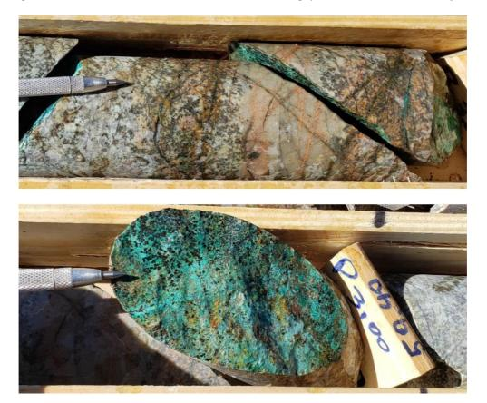
Figure 7: Drill core from hole PNSI22-002 at 59.4m showing quartz-biotite-magnetite veins with Cu-Fe oxides
