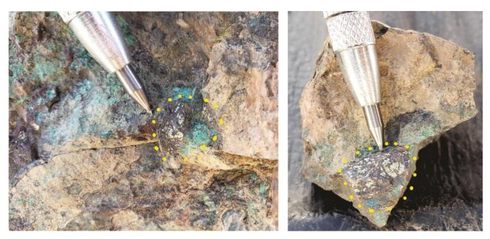
**Figure 5:** Hematite-Specularite sample with Fe, Cu oxidised minerals, and Chalcopyrite cumulates. The dotted points highlight the chalcopyrite cumulates.
