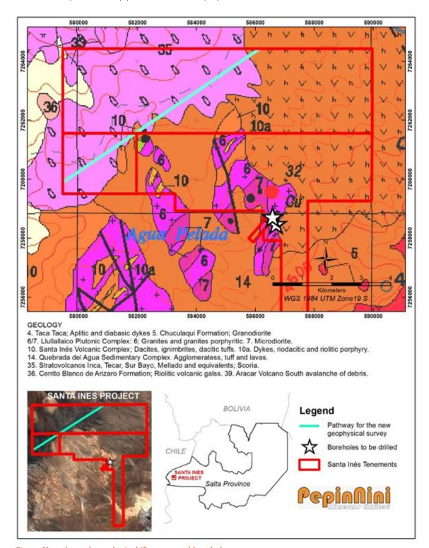
Figure 11 – planned geophysical IP survey and boreholes
