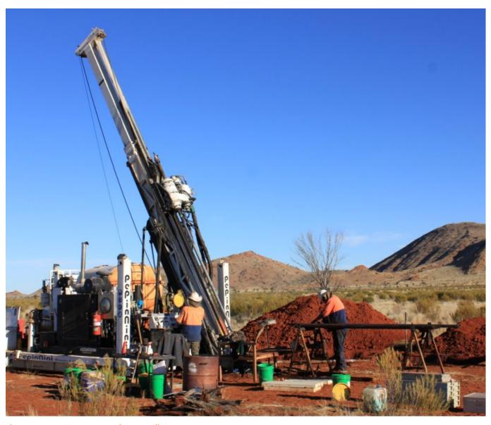
Photo 17 - PepinNini Diamond Core Drilling Rig
