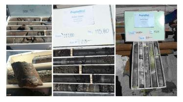
Figure 2 Drill core Borehole PNN-PA-DW-03 permeable sand and sedimentary volcanic breccia
