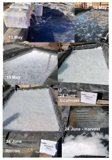
Figure 6 Brine Evaporation Concentration Sequence
