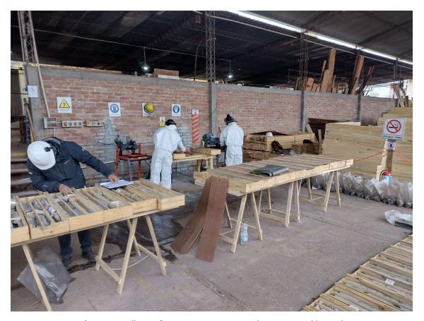
Figure 3: Drill core from Santa Ines project being cut and logged
