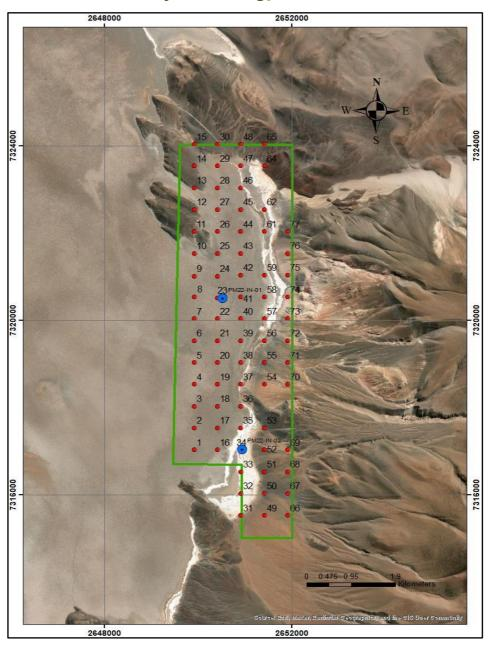
**Figure 1**: Drill hole locations at Incahuasi salar (blue dots) and completed TEM geophysical survey points (red dots) with Sisifo Licence and potential Resource area (green outline).
