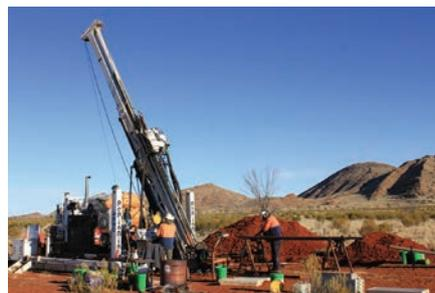
Photo 10: PepinNini Diamond Core Drilling Rig
