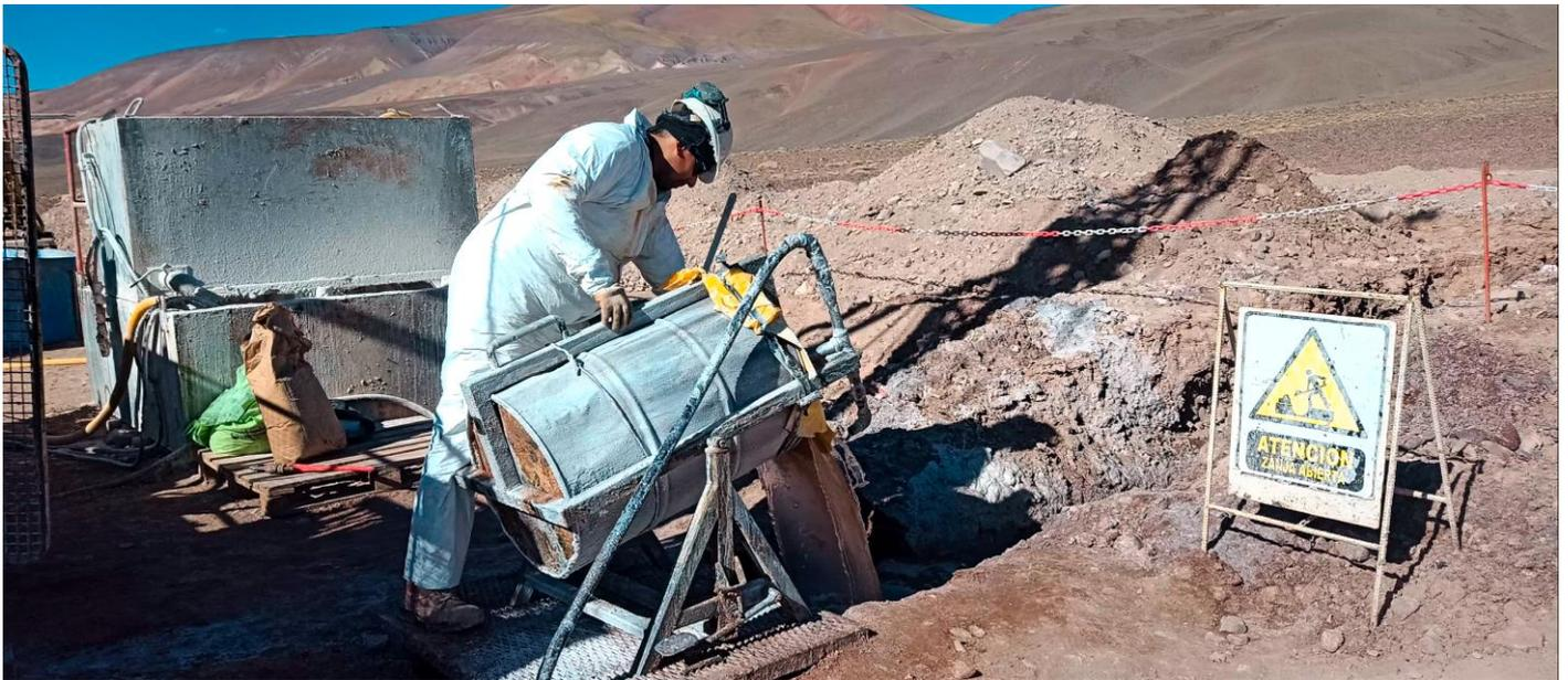
**Figure 5:** Brines packer testing at drillhole PM23-IN-04 at Incahuasi salar, Salta Lithium Project.
