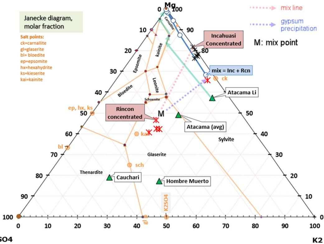
Figure 3 – Phase diagram indicating chemical pathway of the evaporation process
