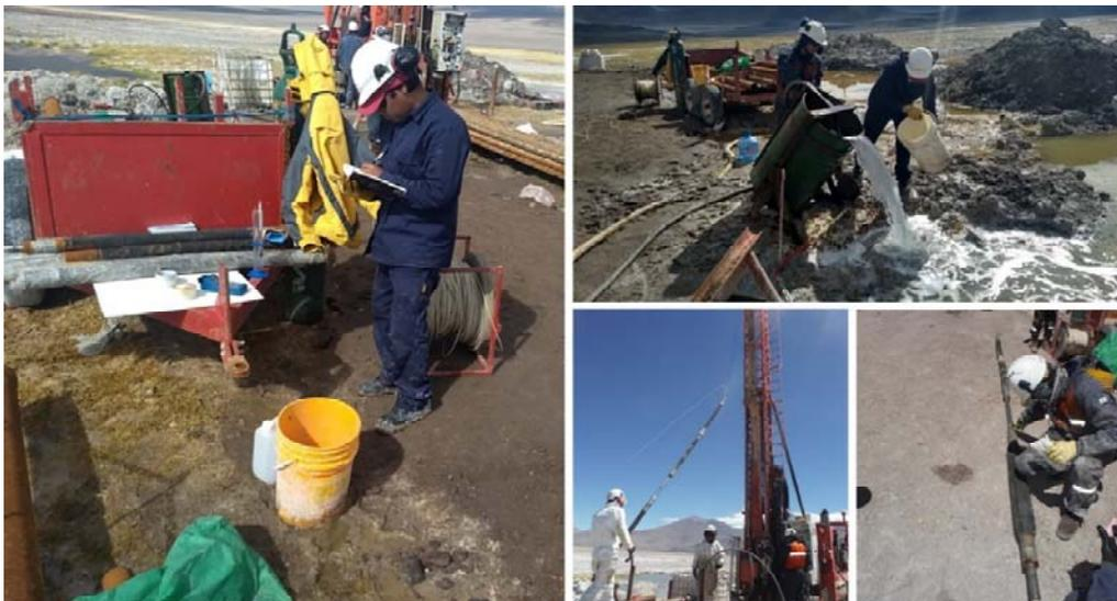
Photo 2 - Brine sampling with packers borehole PNN-SU-DW-01
