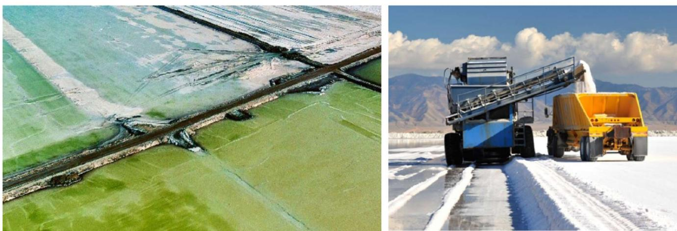
**Figure 8 – Examples of Evaporation Ponds and Harvesting of Concentrate**
