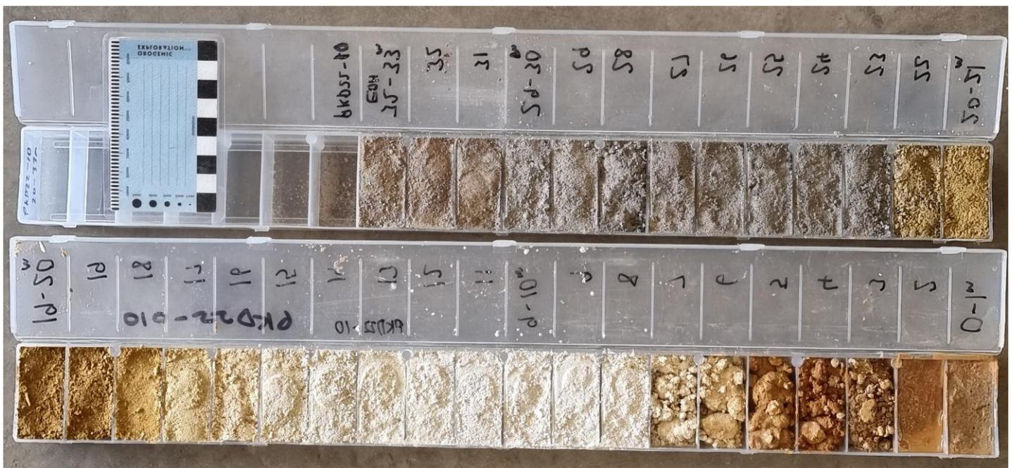
**Image 1:** Chip tray from drillhole PKD22-010 at Eyre Peninsula Kaolin Project.
