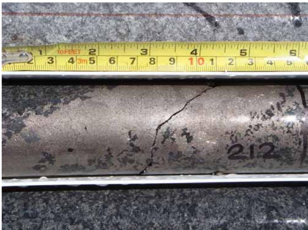
**Borehole DD07HAR008: 211.9 – 212.0m. Massive sulphide mineralisation consisting primarily of pyrrhotite with accessory chalcopyrite and pentlandite. Assays: 0.29% Cu and 0.31% Ni**
