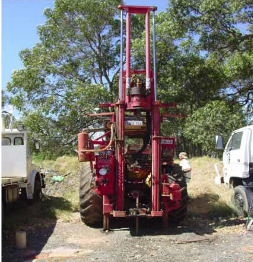
**Company owned Vacuum Drilling Rig**
