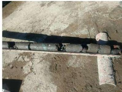
Recovering cores borehole PNN-PA-DW-03
