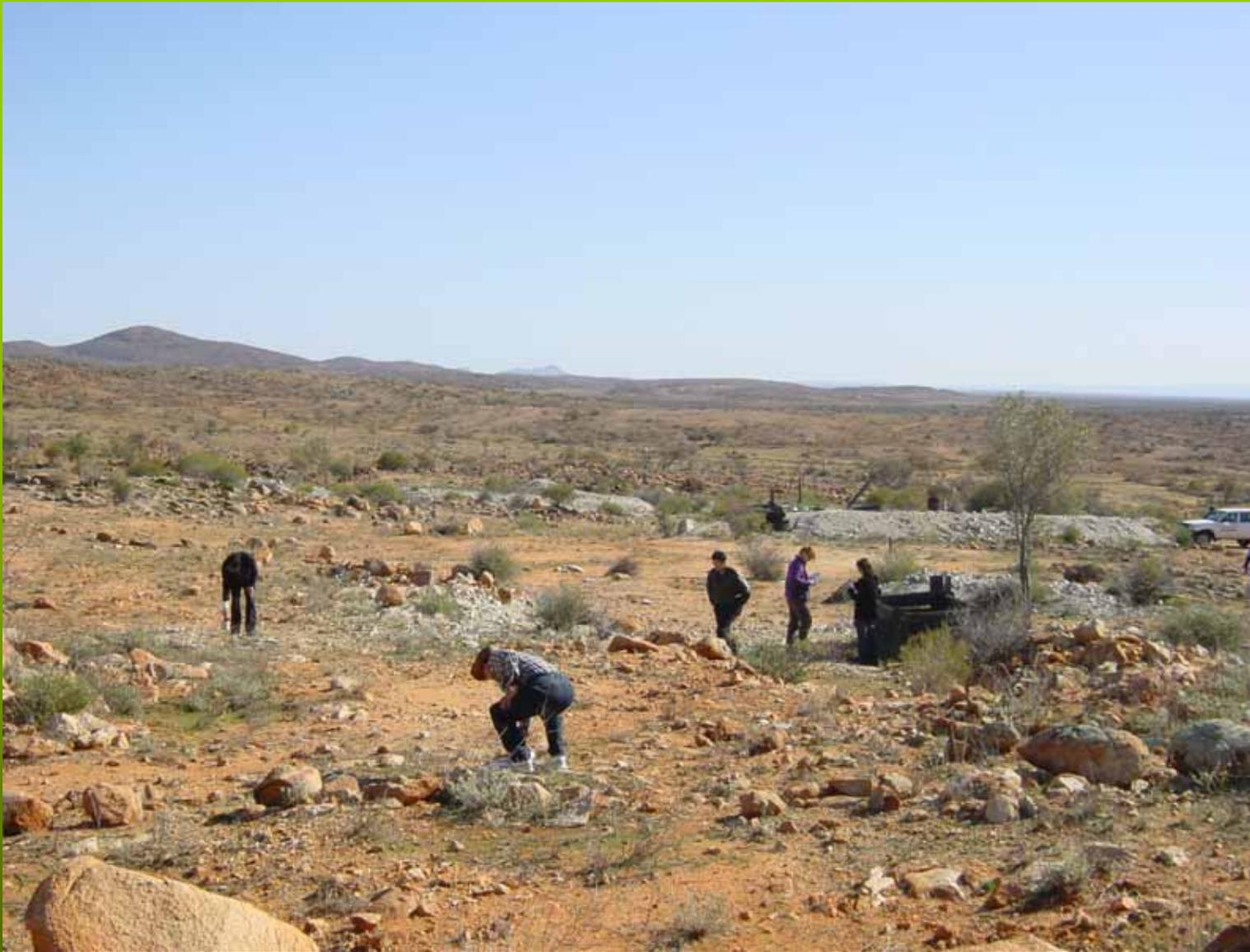
**Mullock heaps beside old shafts contain 100 tonnes of ore grade material – readily available bulk sample for metallurgical testing**
