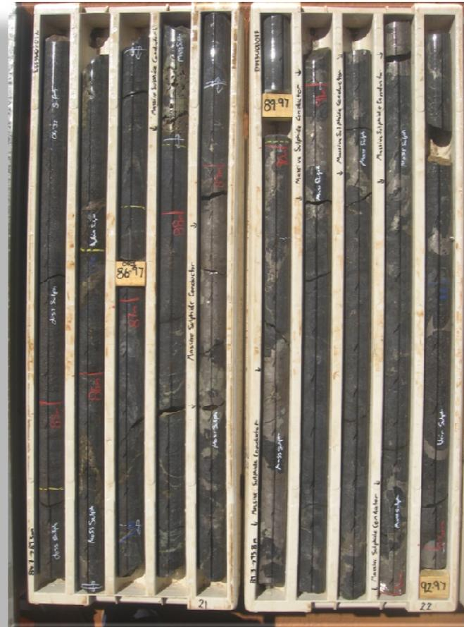
**Significant massive, matrix and disseminated sulphide in ultramafic host rock**
