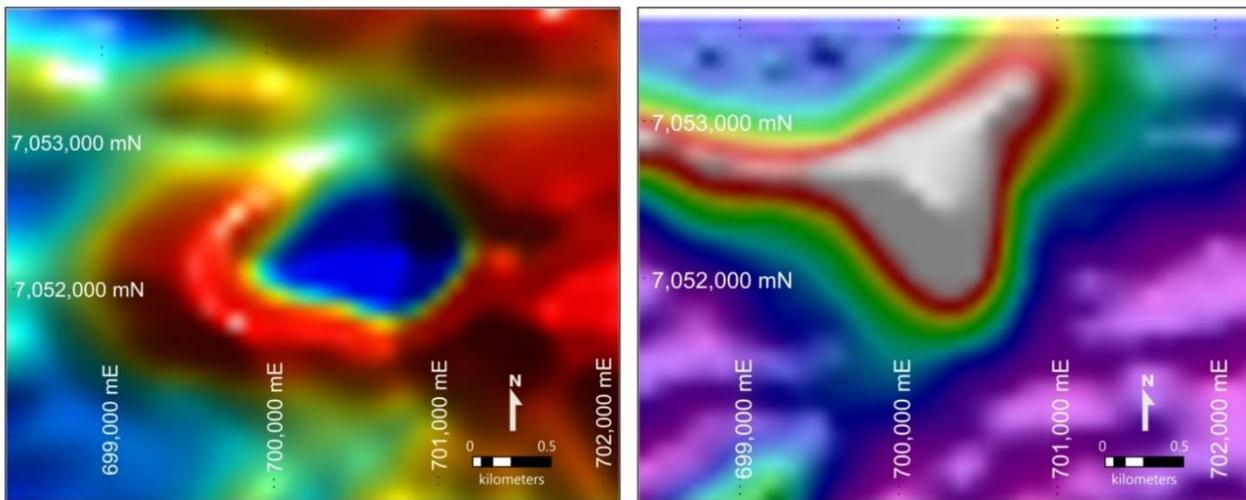
**Figure 2:** Fowler Target – Total Magnetic Intensity(TMI) image (left) and AEM SkyTEM516 image (right) (Z component Channel 35)
