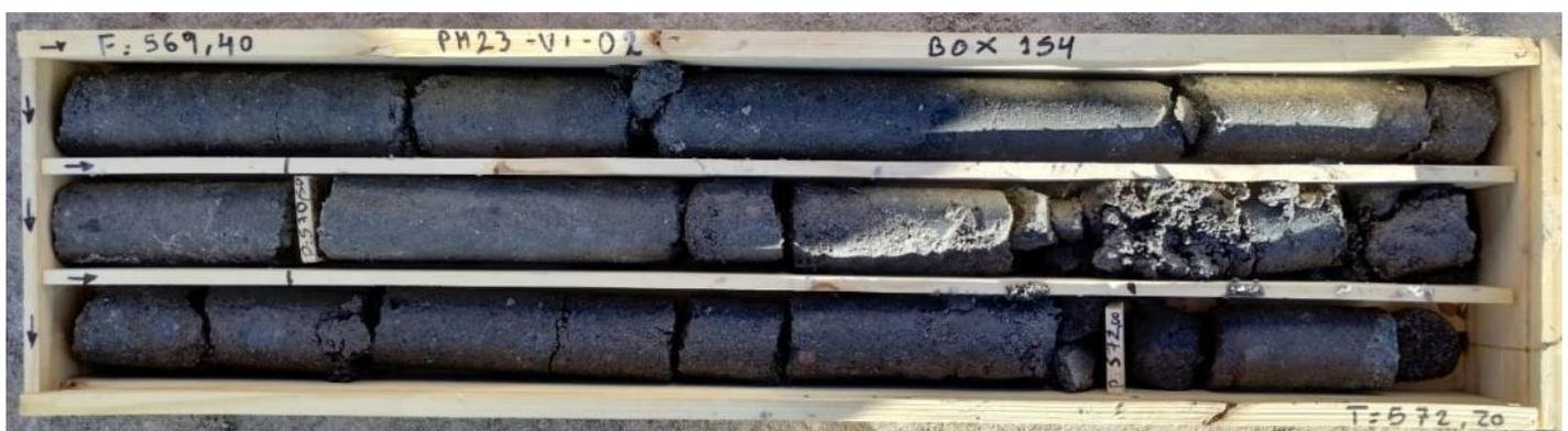
**Figure 3:** Drill core from 569.4 to 572.2 metres depth in drillhole PM23-VI-02 at Rincon salar (Note: high core recovery and sandy matrix)
