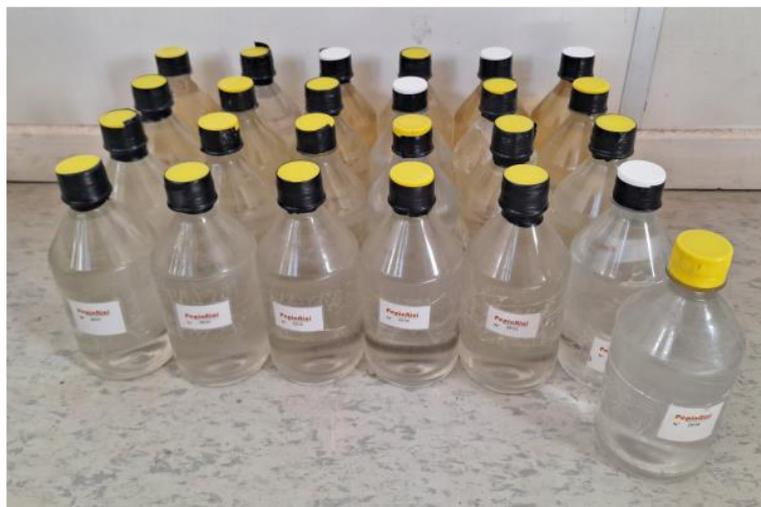
**Figure 2:** Lithium brine samples (500ml bottles) from drillhole PM23-VI-02 sent for laboratory assay tests
