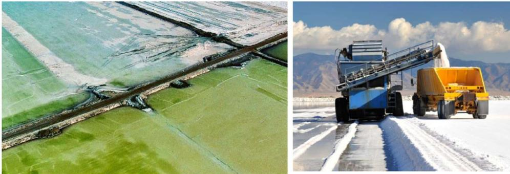
**Figure 6 – Examples of Evaporation Ponds and Harvesting of Concentrate**
