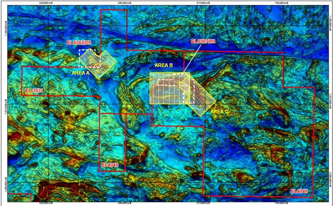
**Proposed orientation SkyTEM survey areas showing 200m orientated flight lines over Hanging Knoll (Area A) and Caroline Intrusion (Areas B and C) on RTP colourdraped magnetic image.**
