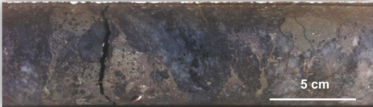
**Figure 4d:** DD12COP013 from depth 160 metres: image showing the mineralogical and textural aspects of a felsic orthogneiss from the Byron Prospect that has been brecciated and milled by remobilised sulphides.
