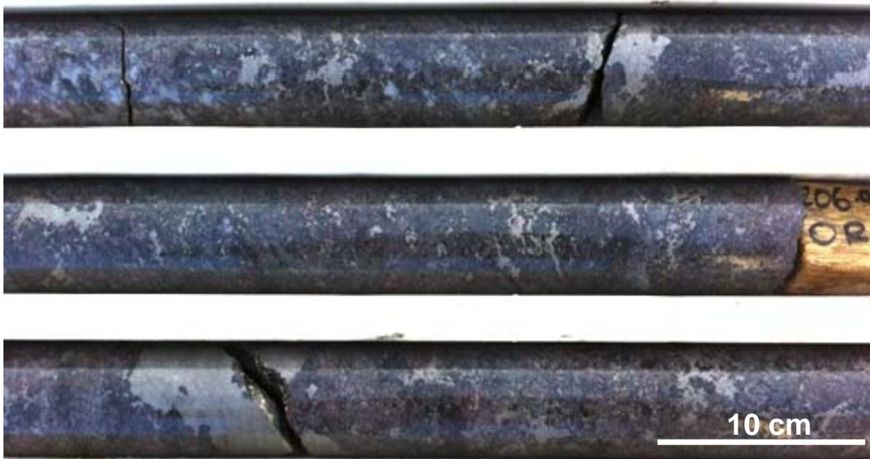
**Figure 4a:** DD12COP008 from depth 205 metres: image showing massive to semi-massive pyrrhotite hosted within a pyroxene+garnet granulite. Lithological comparisons can be made between the rocks from the Byron Prospect to those that host the recently discovered Nova Ni-Cu deposit of Sirius Resources in Western Australia.
