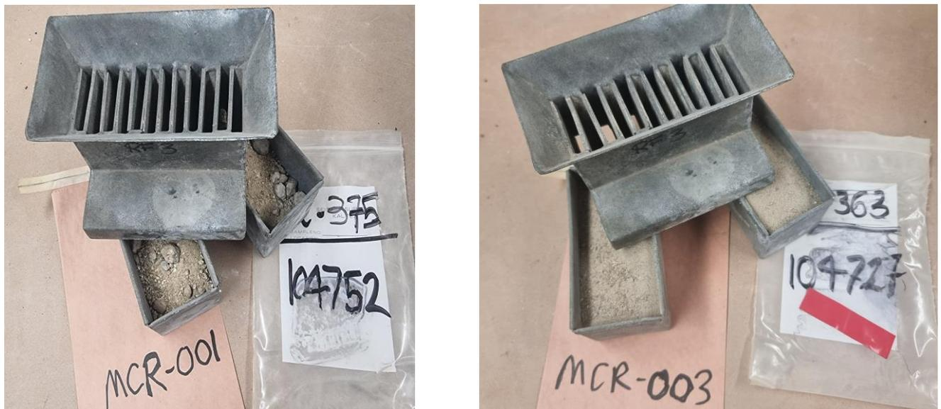
**Figure 1:** Drill sample splitting, Musgrave Nickel-Copper-Cobalt Project, Musgrave province, South Australia
